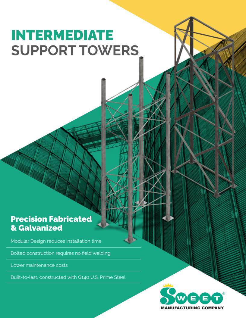
Intermediate towers are steel structures used to support material handling equipment, allow access for maintenance, connections with machinery or with other installations within a facility. Sweet intermediate towers are secure, convenient, and made of precision fabricated U.S. prime G140 galvanized steel for fast and easy modular erection that does not require field welding, painting or field alteration. A hot-dipped galvanized structural steel option is also available.
