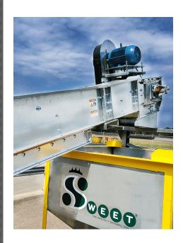
A high capacity corn processing plant approached a Sweet Manufacturing authorized dealer, looking for a Low Profile Conveyor that could fit underneath a bin floor with a low clearance level of 12.75" + slide gates. They were looking for a product that could easily handle 6,000 BPH of corn with low maintenance requirements.
