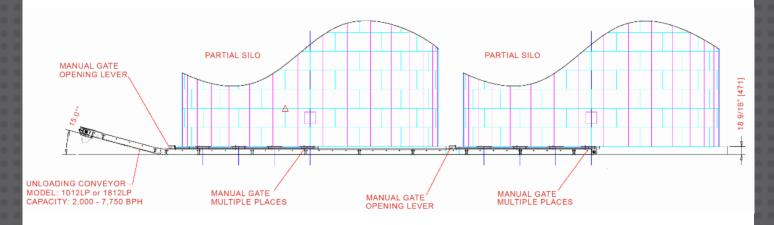
**Built to Perform:** Perhaps the main feature is a 15° curve that allows the conveyor to lay horizontally underneath a bin floor and then curve up to discharge into another piece of equipment. Outfitted with a curved tail, fixed shaft, and UHMW lip seals on the shafts at the head & tail, this small conveyor is designed for installation in tough to reach places. Already seen in applications besides grain bin unloading, this is a versatile conveyor that can handle almost anything you throw in it!
